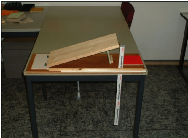
Figure 17: The ramp used to measure the estimated friction coefficients produced by the participants. The ramp had to be adjusted to the angle at which the respective tile would just about start to slide. In the case of skin as reference surface, observers were told to imagine the ramp to be their torso or to be covered with skin.
